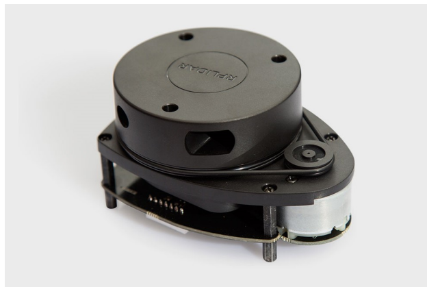
Figure 4.2: The Slamtec RPLIDAR A1 is a 360-degree, two-dimensional lidar with a scanning range of 0.15 to 12 meters, and a 3960Hz sample frequency [42].
